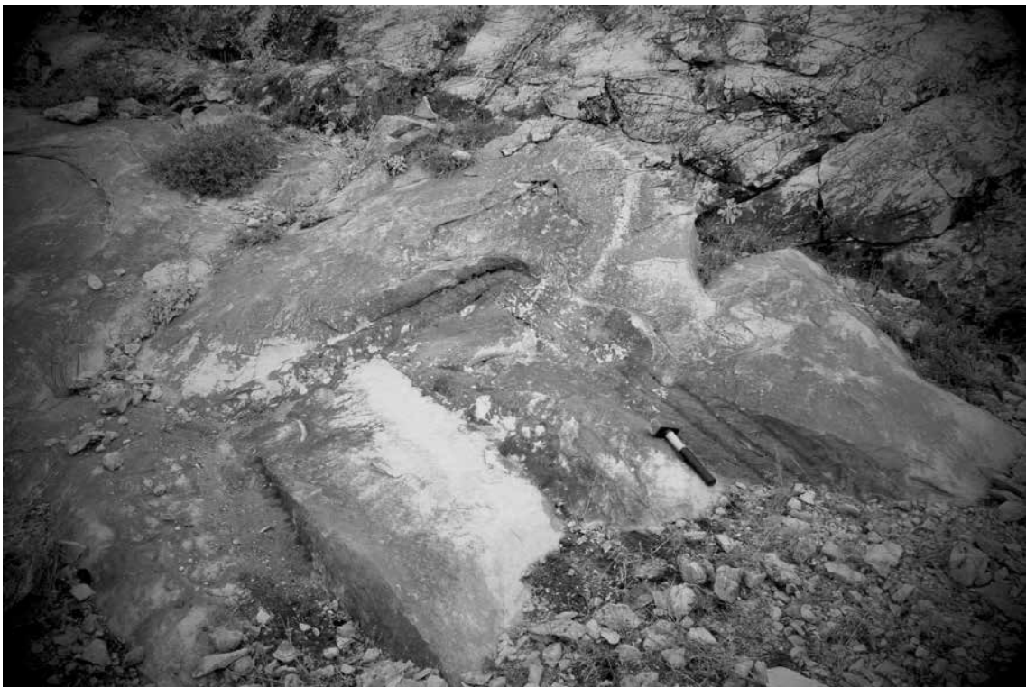
Fig. 9 - Detail of an initial horizontal cut of a quarry channel
